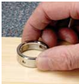
4. An anti-theft thermal ring should be laid on a flat surface with the internal lip uppermost.
