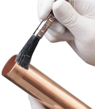
If the complete ring of solder does not appear on heating, apply additional flux to the mouth of the socket and end feed the joint with our N165 (Copper coloured) or N166 (Brass coloured) cadmium-free silver brazing alloy, or an equivalent to the compositional requirements of BS EN 1044 AG103 (formerly BS 1845 AG14).
