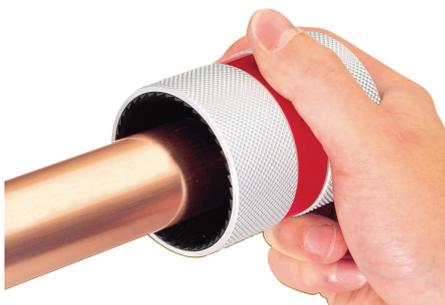
**3.** Clean the inside of the fitting socket and the outside of the tube with a Yorkshire cleaning pad, fine sandpaper or steel wool.
